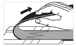
After cooling remove tape from guide rail
