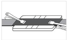
Position the covering plate and fix it with clamps
