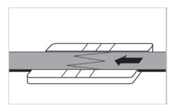
Place the prepared tape ends into the guide rail
